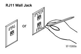
The RJ11 6-pin jack uses the center two pins. For pin assignments, refer to *Cables & Connectors* on page 14.
